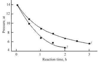
**Fig. 1.** Change of acetylene pressure in the course of 1,4-butanediol (**Ie**) vinylation: *1*, in the presence of KOH, 7 mol%, *2*, in the presence of CsF–NaOH, 7/7 mol% (reaction temperature 150–158°C).
