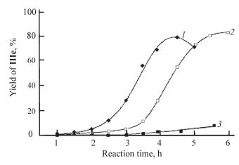
**Fig. 2.** Vinylation of 1,4-butanediol (**Ie**) at atmospheric pressure of acetylene in the presence of a superbasic system CsF–NaOH–DMSO. (*1*) CsF–NaOH 30/30 mol%; (*2*) CsF–NaOH 20/20 mol%; (*3*), CsF–NaOH 10/10 mol%.
